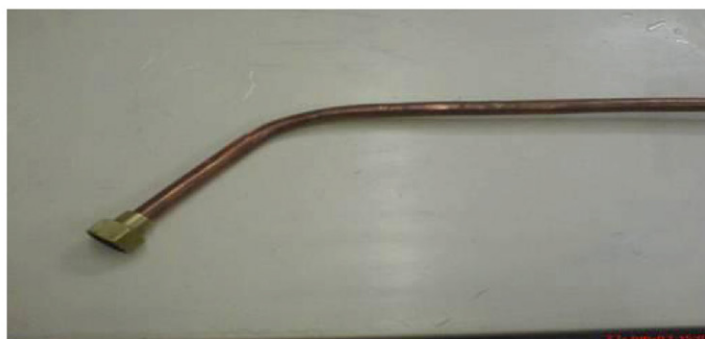
(E) Copper pipe condenser
